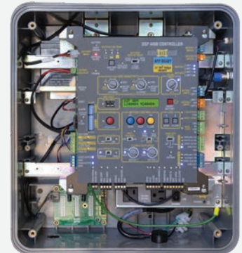
ARM CONTROLLER BOX Heavy-Duty composite plastic enclosure
