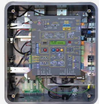
ARM CONTROLLER BOX Heavy-Duty composite plastic enclosure
