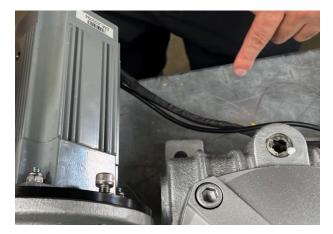
**8** While the motor is still loose make sure the motor cables face towards the gearbox.
