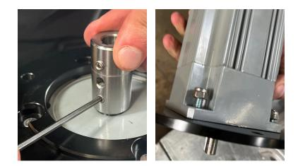
6 Mount the MX053-2 (square motor) into the gearbox aligning the coupler with the key way side up to seamlessly unite both flanges.
