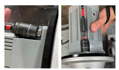
**10** Finally tighten the lock nuts on the 4 corners of the MX053-2 (square motor) to complete the installation. You are all set.
