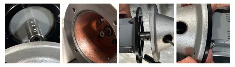
7 Though the open hole of the gearbox, tighten the key way screws with the Allen key, then with your finger, turn the other side of the coupler up and tighten the screws.
