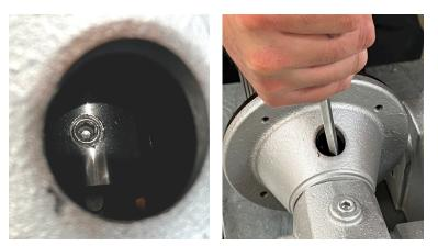
**3** Through the open hole, loosen the 2 set screws on the coupler.
