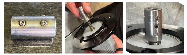
First, tighten set screw on the key way side, then tighten
