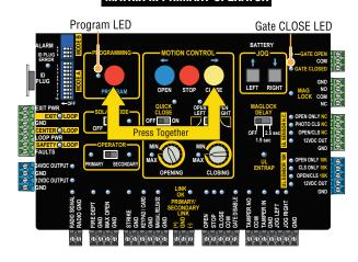
After the final close positions are chosen, press the PROGRAM button again to record the current gate positions for both primary and secondary gates as the virtual CLOSE limits. The PROGRAM LED will turn OFF, the GATE CLOSE LED will turn ON and stay on and the beeping will stop. Virtual CLOSE limits are programmed for both primary and secondary gates.
