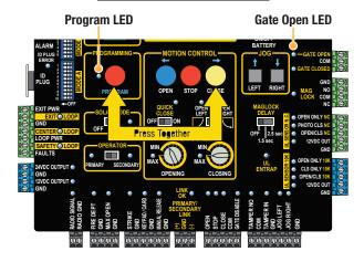
After the final open positions are chosen for both primary and secondary gates, press the PROGRAM button again to record the current
