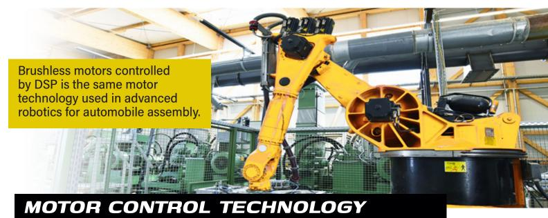
Maximum Controls' brushless dc motor control enables precision movement that traditional brushed motors can not replicate. For example, no overcoasting. This ability is crucial in bi-parting slide gates on the same track, as well as catch posts or columns that can't be avoided.
