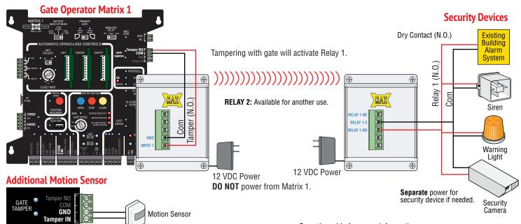
If a motion sensor is added to the Tamper IN input, when the motion sensor gets triggered, security device that is wired to Tamper NO - RELAY 1 will activate (see above).
