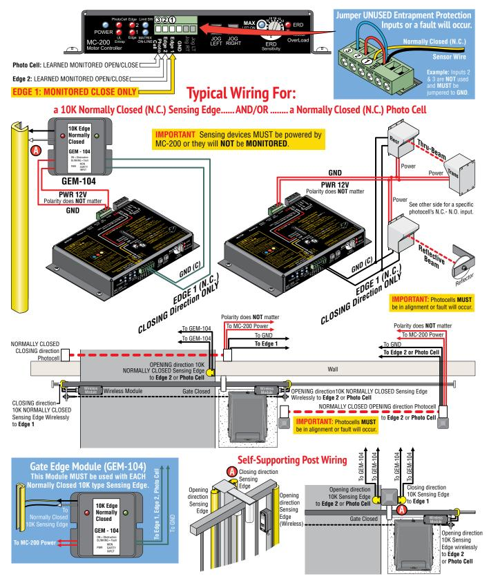
DUAL GATE OPERATORS NOTE: Connect EACH photocell/sensing edge to the corresponding gate operator. See page 10 in the manual.
